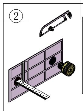
Measure the depth of the inner thread of cold & hot water pipes and mark it.
