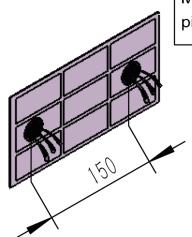
Make sure the middle distance btw the two pipes are 150mm,and allow 5mm adjustment.
