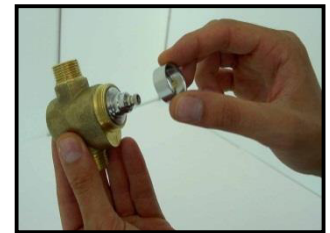
4 - remove the inner ring nut
