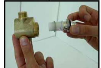
6 - remove and replace the cartridge
