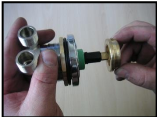
15 - unscrew the brass nut
