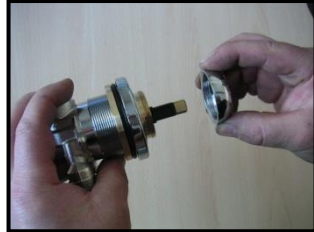
14 - unscrew the ring chromed cover-nut
