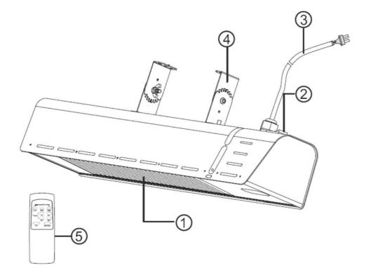
ÿ Front panel with aluminum grille ÿ ON / OFF main power switch ÿ Power cable ÿ Brackets for wall or ceiling mounting ÿ Infrared remote control
