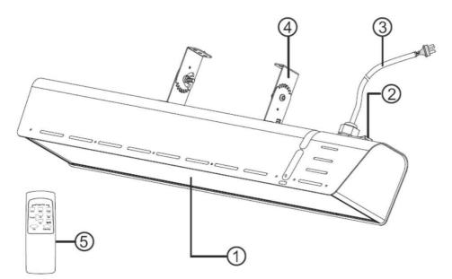
ÿ Black ceramic glass panel ÿ ON / OFF main power switch ÿ Power cable ÿ Brackets for wall or ceiling mounting ÿ Infrared remote control
