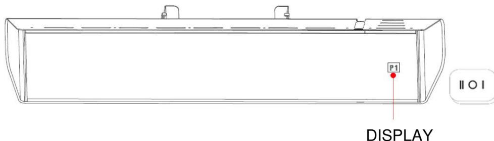
• Connect the heater to a 230-240V ~ 50-60Hz power socket. Set the switch a rocker in position I: the heater starts operating. Attention: The remote control cannot operate the heater at this stage.
