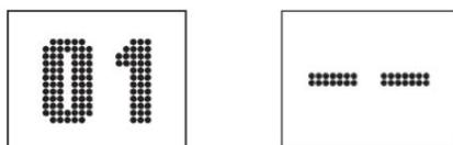
To set the 13 hour timer, point the remote control directly at the receiver and then press 1 2 4 6 on the remote control, "13" will be indicated on the display area. This will cause the heater to automatically enter Standby mode after 13 hours of operation. Once in Standby mode, the "- -" symbol will flash.
