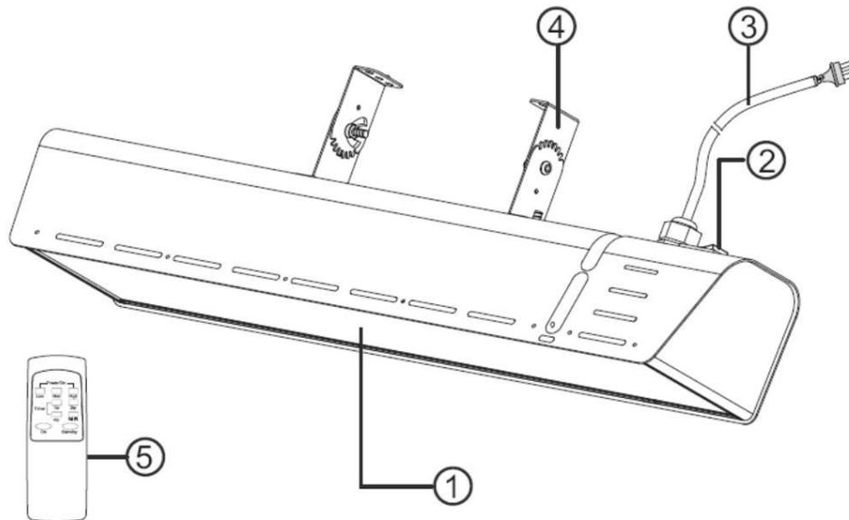
• Black ceramic glass panel • ON / OFF main power switch • Power cable • Brackets for wall or ceiling mounting • Infrared remote control
