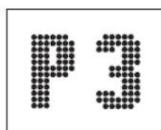
Press the "LOW", "MED" and "HIGH" buttons on the remote control, the heater works with the settings of power LOW and MED, HIGH, and the symbol "P1" "P2" "P3" will be indicated on the display area.
