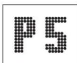
Press "LOW", "MED" and "HIGH" on the remote control, the heater works at LOW and MED, the HIGH power setting and the symbol "P1" "P3" "P5" will be indicated in the display area.
