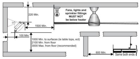
Minimum distances for mounting the heater parallel to the ceiling.
