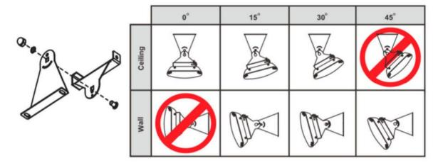
7. Hang the heater from the brackets and secure it securely in place with the mounting bracket locking plates tightening the bolts.
