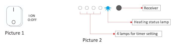
3. Point the remote control directly at the receiver, press the "ON" button, the appliance will emit 1 beep. The device starts to heat up in high power mode (100% of the nominal power), the heating status check bulbs will turn red (figure 3).
