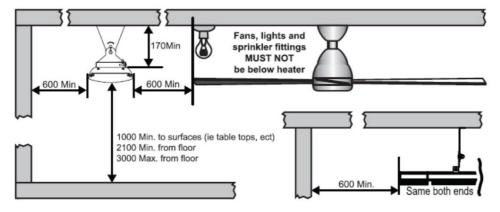
Minimum clearances when mounting the heater at an angle to the ceiling.
