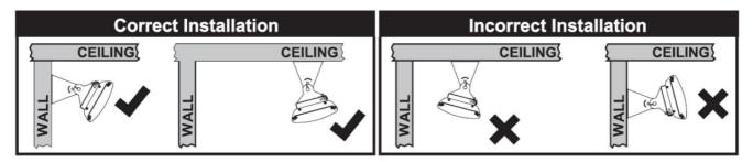
Attention: The heater must never be installed in a position facing upwards or inwards, the heating surface must always be positioned in such a way as to direct the heat downwards or outwards.
