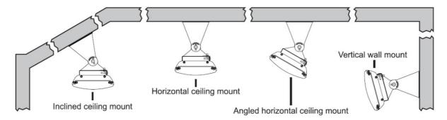
The ideal mounting position is directly above the area to be heated in a longitudinal orientation and facing vertically downwards. If this is not possible, the heater (s) can be mounted on a wall and angled downwards.
