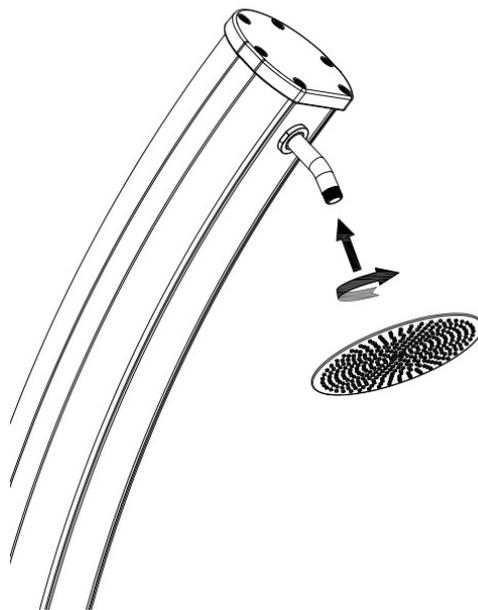
Make sure the rubber washers are positioned correctly before installing the showerhead.
