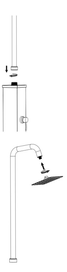
Make sure the rubber washers are positioned correctly before installing the showerhead and top tube.
