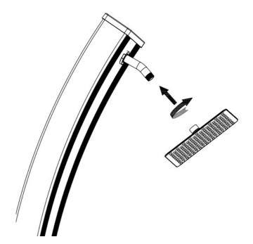
Make sure the rubber washers are positioned correctly before installing the showerhead.
