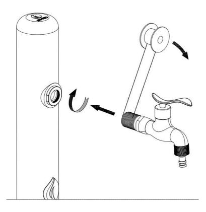
Before installing the tap, ensure that the rubber washer is correctly positioned.
