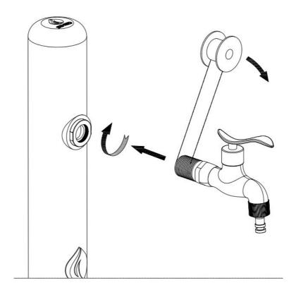
Before installing the tap, ensure that the rubber washer is correctly positioned.
