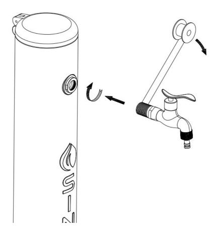
Before installing the tap, ensure that the rubber washer is correctly positioned.
