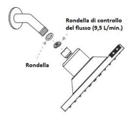
If more pressure is desired, the flow control washer can be removed.
