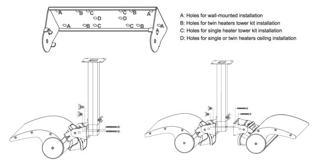
4. 4. Attach the bracket to the ceiling using dowels adapted to your application (not included).
