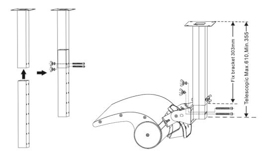
NOTE: The minimum distance between the bottom end of the pole and the ceiling is 35.5 cm and the maximum distance is 61 cm. Refer to the Site Selection section to ensure that all minimum distances have been observed.
