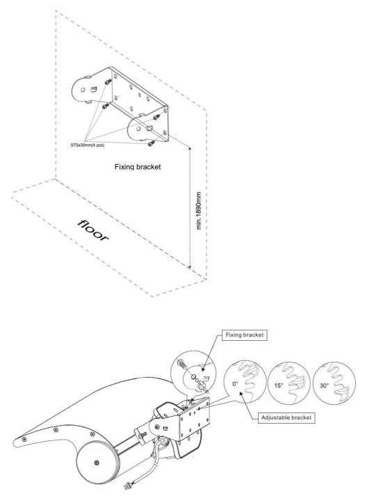
2.2.4. Attach the bracket to the ceiling or wall using dowels or fasteners suitable for your application (not included).
