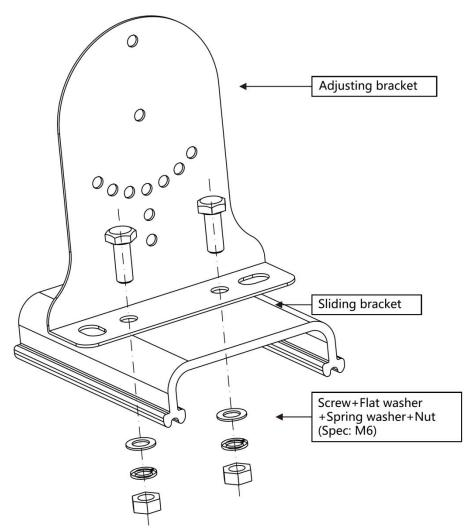
Step 2: Installation of sliding bracket & heater, as arrow points.
