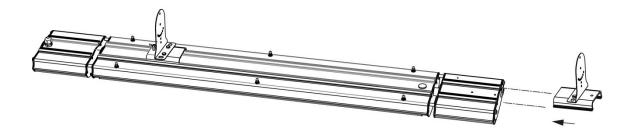
Step 3: Fix adjusting bracket into the wall by expansion screws.Installation of two adjusting brackets; make sure lock brackets tight by butterfly hand screw.
