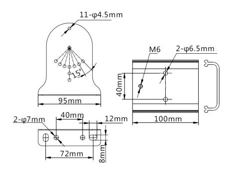
Step 1: Installation of adjusting bracket & sliding bracket.
