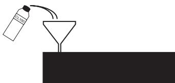
Warning: Make sure that the liquid does not flow outside the filling-opening. In case liquid has been spilled outside the filling opening, make sure this is dried up before lighting the fire.
