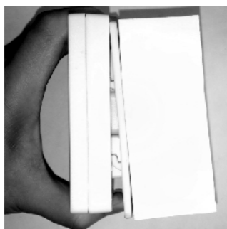
3. Clamping the controller and installation board together correctly.
